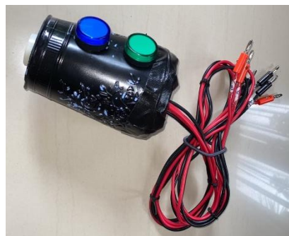
Gambar 7. Indikator pengingat alat smart safety belt
